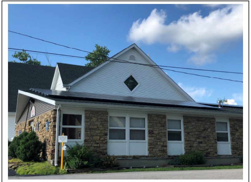
The solar panels in the above example should have been installed in a much less conspicuous location. The tangle of wires leading down from the panels is also not consistent with these design guidelines. The panels on the Nashville, Indiana church below are much more appropriately installed and are almost invisible at street level.
